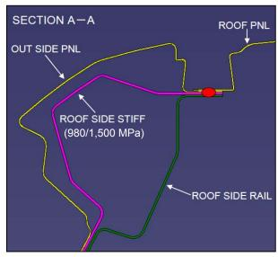
Roof Panel Section A - A
