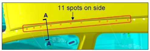
Roof Panel 4-Plate Spot Weld Area
